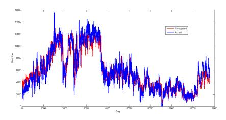
Figure 5: Gas flow forecast of cross border node 3 - 3 months. RMSE: 1312
