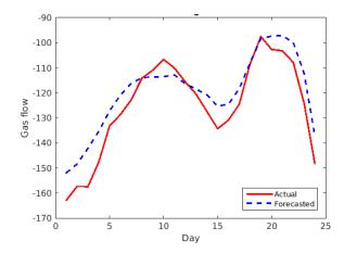
Figure 3: 24-hours gas flow forecast of node 2 - RMSE: 8
