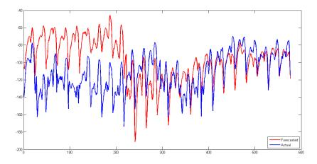
Figure 4: Hourly gas flow forecast of node 2 using the trained network and live data - 3 months. RMSE: 32  $\,$
